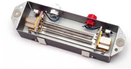
Figure 2.3: Spring Reverb Unit [Ashley Pomeroy CC BY-SA 4.0]
